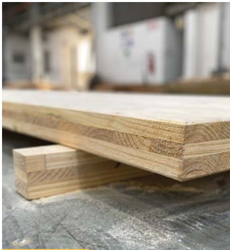
Cross-laminated timber (CLT) panels in profile.
