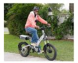
power on demand, with a maximum speed of 25km/h (15.5mph) and has a range of up to 65 km. The electric bicycle was provided by Cycology.
